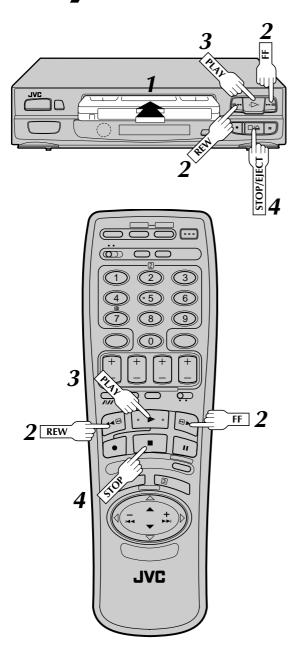
The easiest, most basic operation possible with your video recorder is tape playback. Already-recorded signals on a video tape are read by your video recorder and displayed on your TV just like a TV programme.
